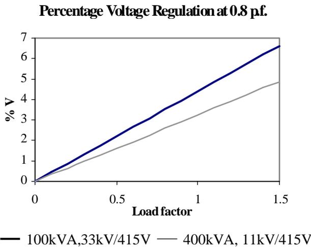
Figure 4.1 – Percentage Voltage Regulation at 0.8 p.f.
