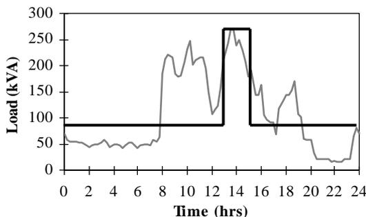
Figure 3.3 - Daily Load Profile of Industrial Load
