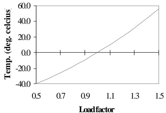
**Figure 3.1** – Excess in Hotspot temperature with load factor
