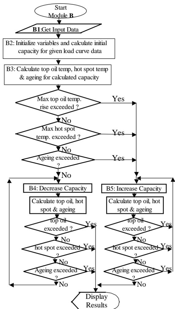
Figure 2.2 - Flow Chart for finding Optimum Transformer Capacity
