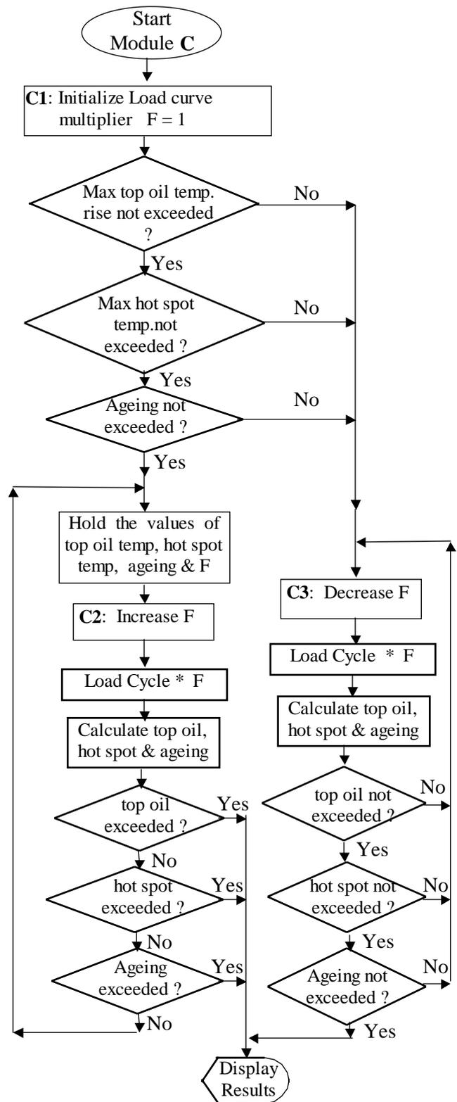
**Figure 2.3** - Flow Chart for finding Optimum Load Curve Multiplier
