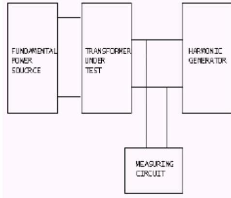
Figure 1 – Harmonic Load Test Arrangement
