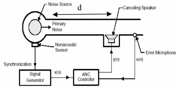
Fig. 4 Narrowband Feedforward ANC System
