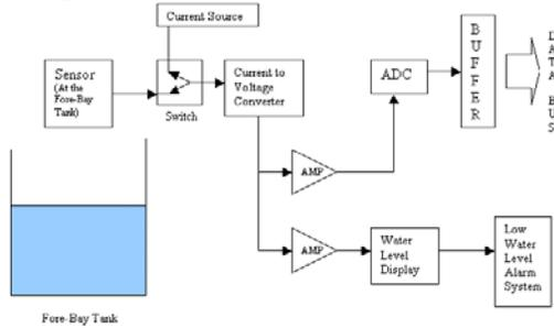
Figure 3: Block Diagram of the Water Level Sensor
