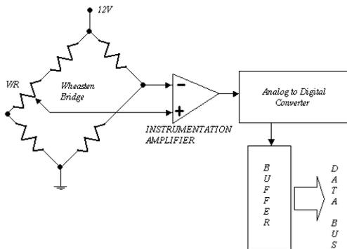
Figure 4: Block Diagram of the Valve Position Sensor
