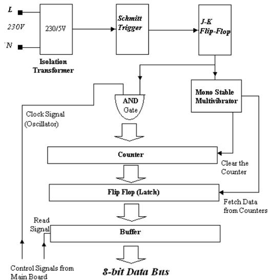
Figure 2: Block Diagram of the Frequency Counter
