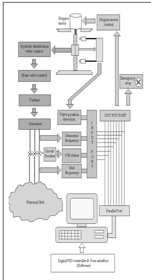
Figure 1: Basic Block Diagram of the System
