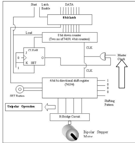
Figure 5: Stepper Drive Control Block Diagram
