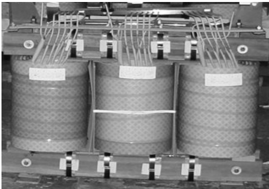
Figure 1 – Core-winding assembly ready for ovening
