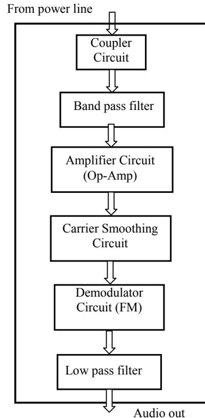
**Receiver circuit functional block diagram**
