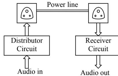
The power line based intercom system consist two basic circuits and they are Distributor and Receiver circuits. Distributor circuit is used to modulate our signal into frequency modulated form and to change our modulated carrier signal into desired form. Receiver circuit is used to demodulate our modulated carrier signal which is received from the power line and to filter our audio signal noisy signal.
