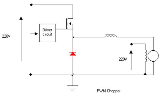
Fig: 4.3 Basic (Class A) Chopper circuit
