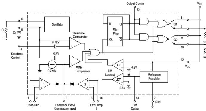
Fig 2. Control IC Internal Arrangement
