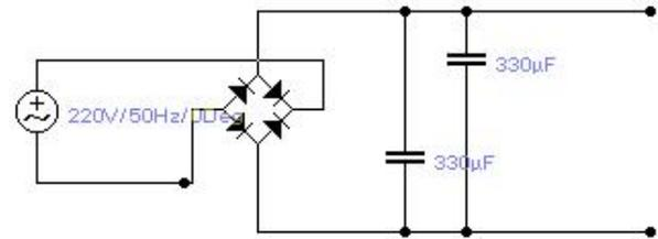
Fig 4. Bridge Circuit
