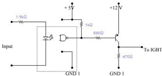
Fig 5. Isolation Circuit
