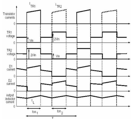
Fig. 2 Push-Pull Waveforms
