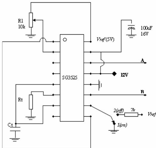
Fig. 3 PWM Controller Circuit
