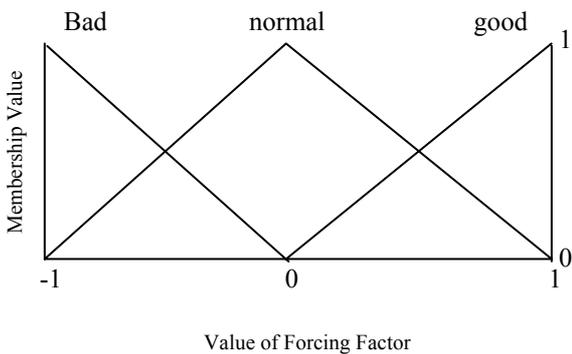
Fig.6 Membership function of the leadership, communication, unity, which has three fuzzy sets and used in RULE 1 to 9
