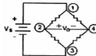
Fig 1: Force Sensor(FS) series circuit
