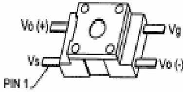
**Fig 2: Sensor Pinout**
