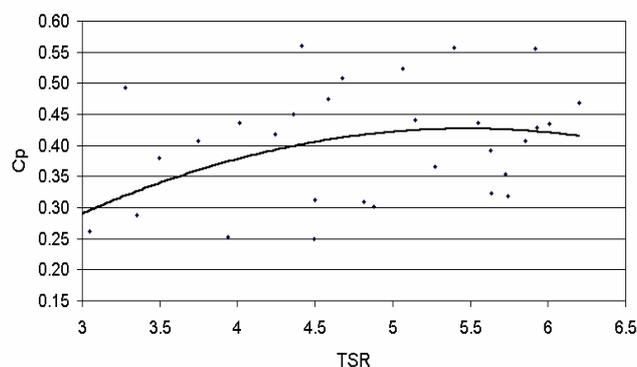
Fig. 1 Coefficient of Performance ( $C_p$ ) Vs. Tip Speed Ratio (TSR)
