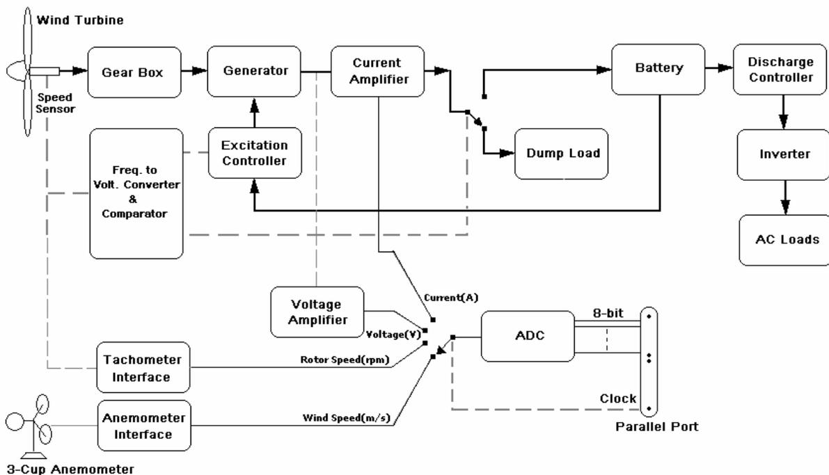
Fig. 7 Block Diagram of Windpro Wind Turbine
