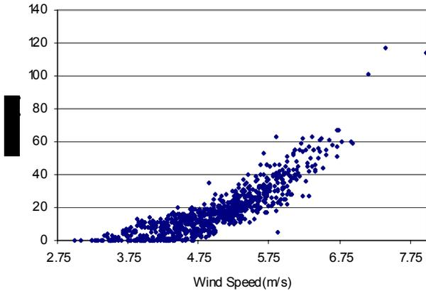
Fig. 6 Power output Vs wind speed curve
