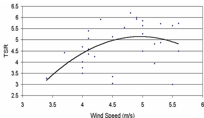
Fig. 2 Tip Speed Ratio (TSR) vs. Wind speed
