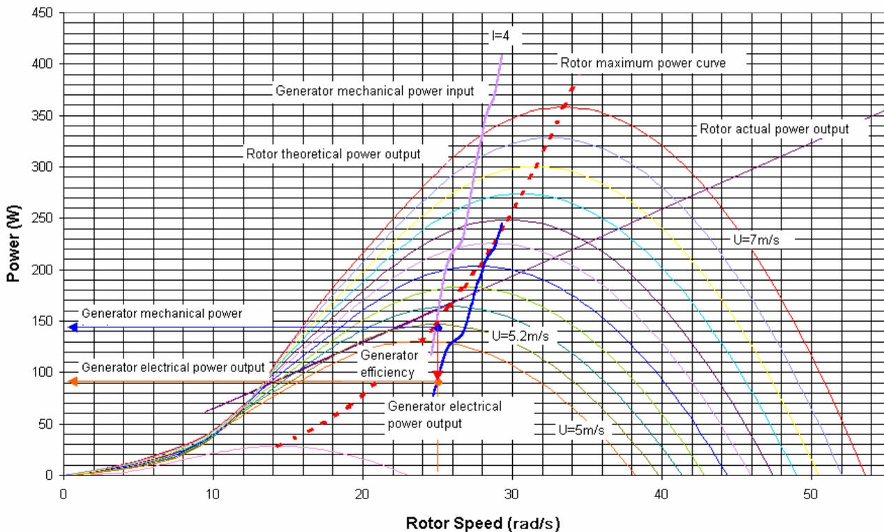
Fig. 5 Rotor mechanical power and generator input/output power as a function of rotor speed
