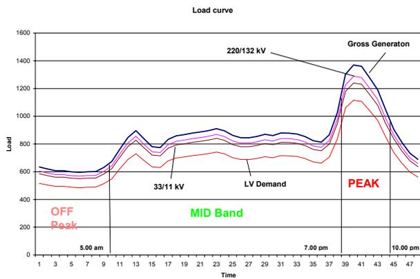
**Figure 1: Demand Profile considering losses at each voltage level**
