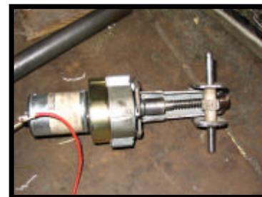
**Figure 4: Motor, Gear train & Worm wheel**
