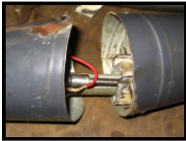
**Figure 5: Motor, Gear train & Worm wheel**
