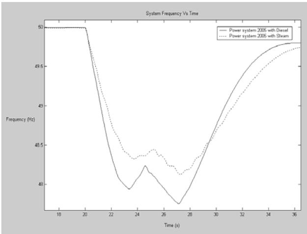
Fig. 4 Comparison of frequency plots of same contingency of system of 2005 with diesel engines and them being replaced with steam turbines.
