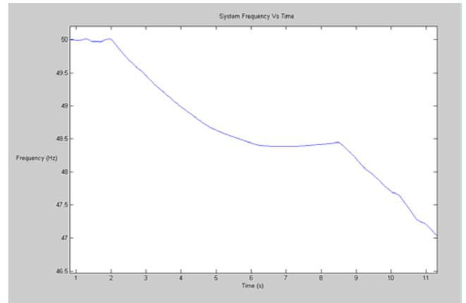
Fig. 6 Frequency plot of the total system failure occurred on 25/01/2004.
