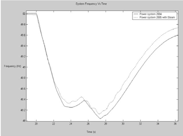
Fig. 3 Comparison of frequency plots of similar contingencies of systems of 2003 and 2005 with diesel engines replaced with steam.
