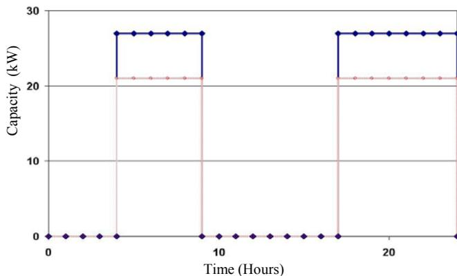
Fig 3: Expected Load Curve for 27kW Option
