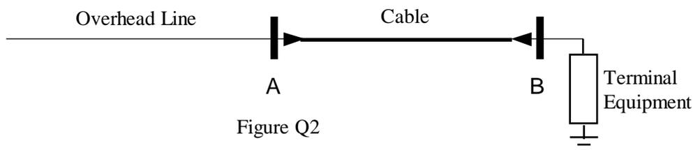
If a triangular voltage surge (vertical front, 200 kV peak decaying to zero in 40 μs) originates in the overhead line and arrives at A at time t = 0, determine using the Bewley Lattice diagram, and sketch the voltage variation at A and B for the first 25μs. [18 marks]
