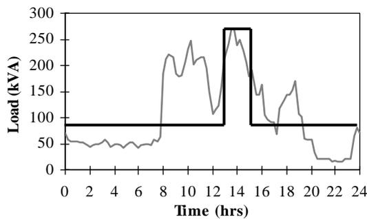
Figure 3.4 - Daily Load Profile of Industrial Load
