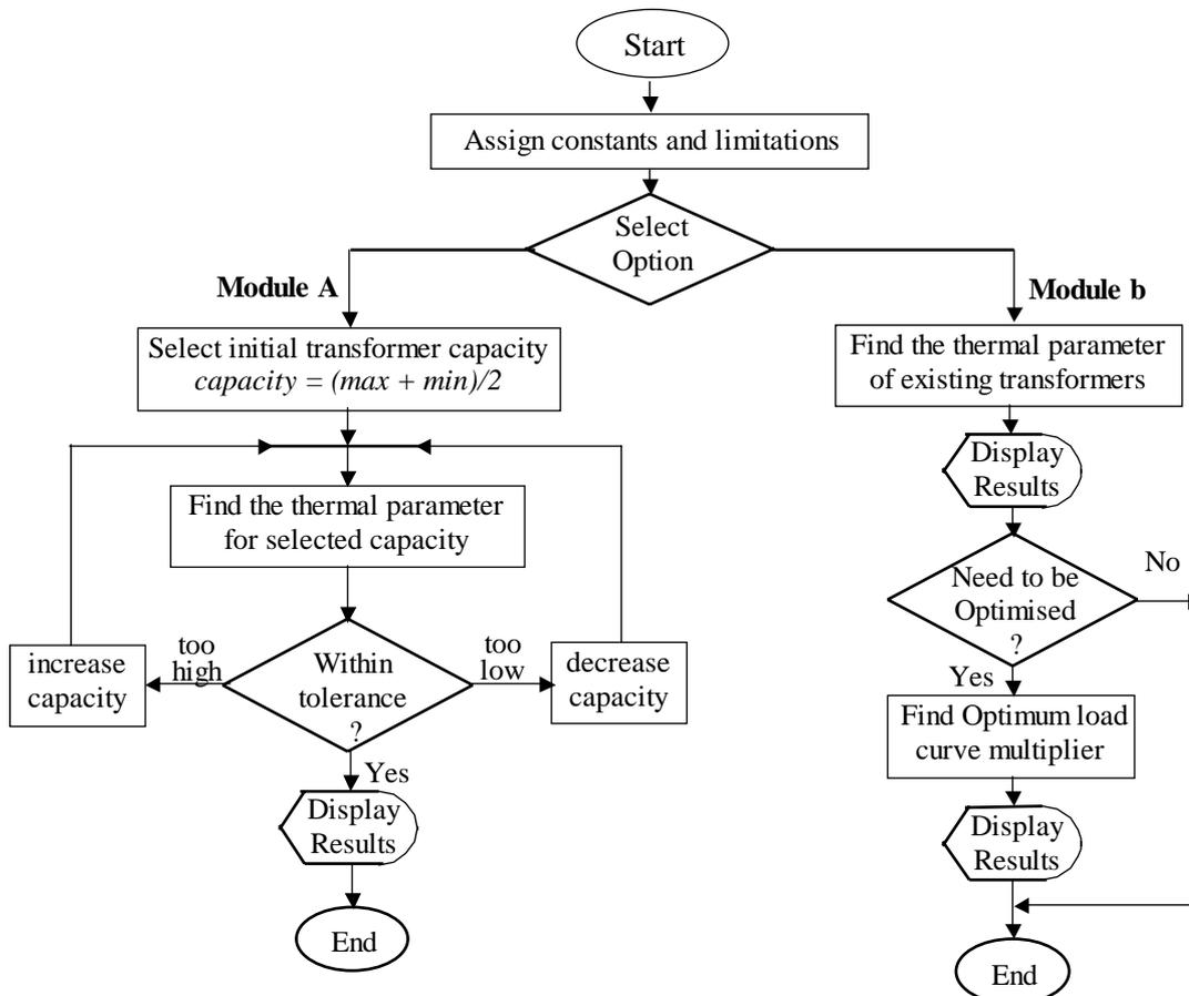
Figure 3.1 - Flow Chart for thermal parameters
