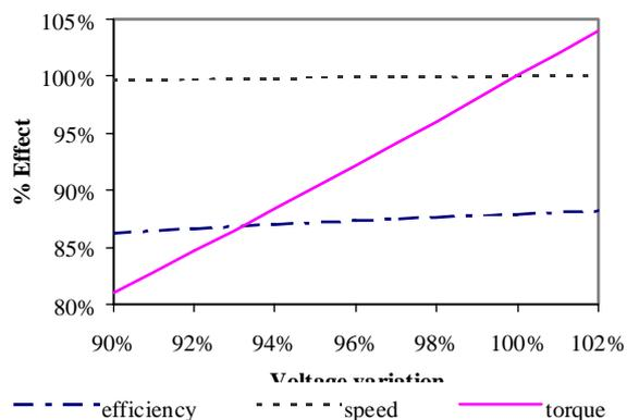
Figure 4.5 – Variation of motor performance with reduction in terminal voltage
