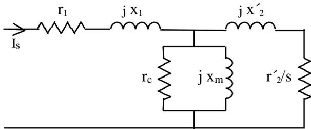
Figure 4.2 - Equivalent circuit used for the induction motor
