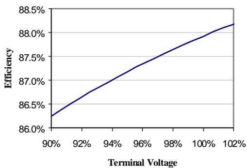
Figure 4.4 - Variation of full-load efficiency with a reduction in terminal voltage
