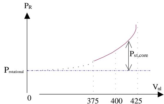
Figure 4.3 - Variation of rotational loss with voltage
