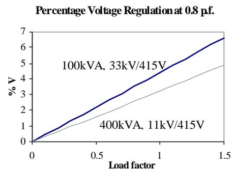
Figure 4.1 – Percentage Voltage Regulation at 0.8 pf
