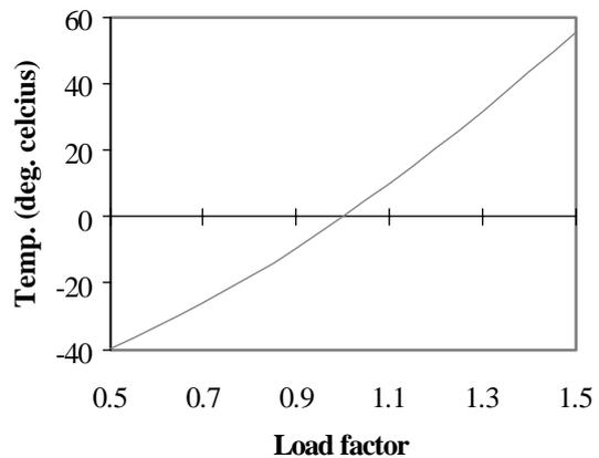
**Figure 3.3** – Excess in Hotspot temperature with load factor
