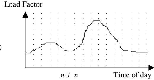
Figure 3.2 Load Curve
