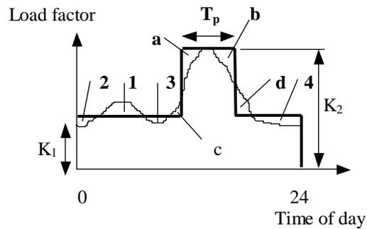
Figure 2.1- Two-Step Approximation method
