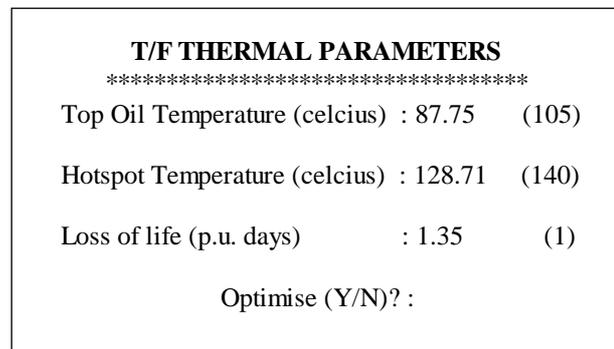
Display 3.1 - Thermal parameters of existing transformer at the Industrial Load
