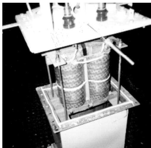
Figure 7 - Single phase coconut oil filled transformer
