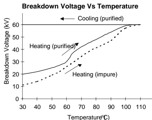
Figure 1 - Heating/Cooling Curve of Coconut Oil
