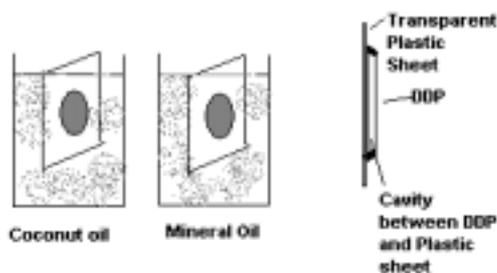
Figure 6 - Oil Impregnation Test
