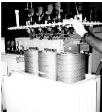
Figure 9 - Three phase coconut oil filled transformer
