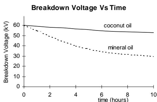
Figure 2 - Degradation due to moisture absorption
