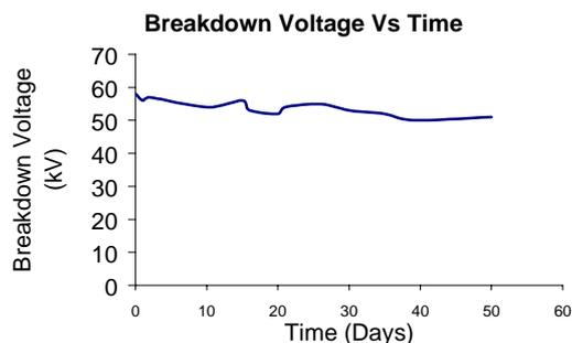
Figure 4 - Degradation of oil due to small leak
