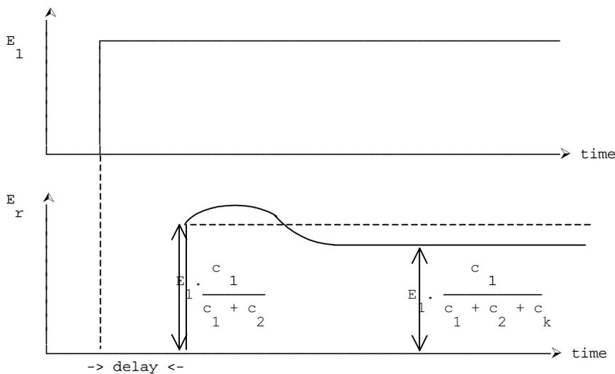
Figure 6.22 - Waveforms for simple capacitor connection
