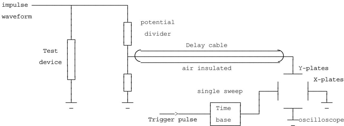
Figure 6.14 - Observation of impulse waveform through potential divider
