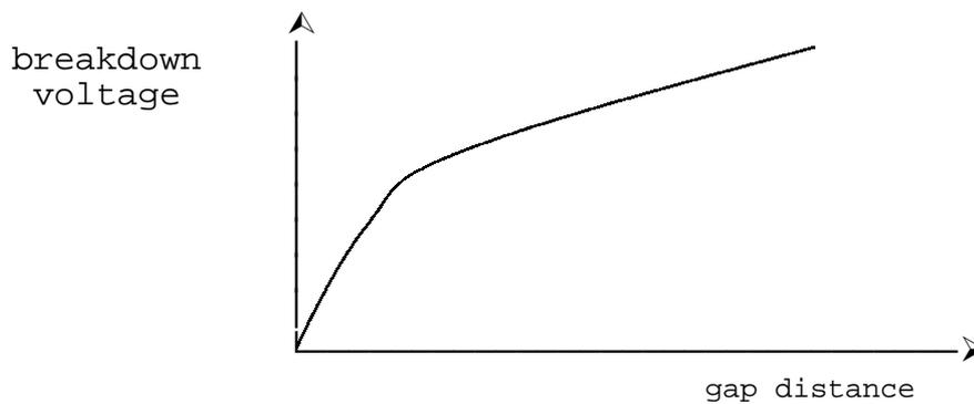
Figure 6.3 - Breakdown voltage characteristic of sphere gaps
