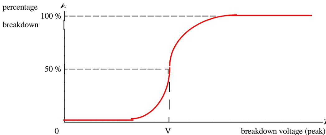
Figure 6.6 - Breakdown voltage characteristic for impulses
