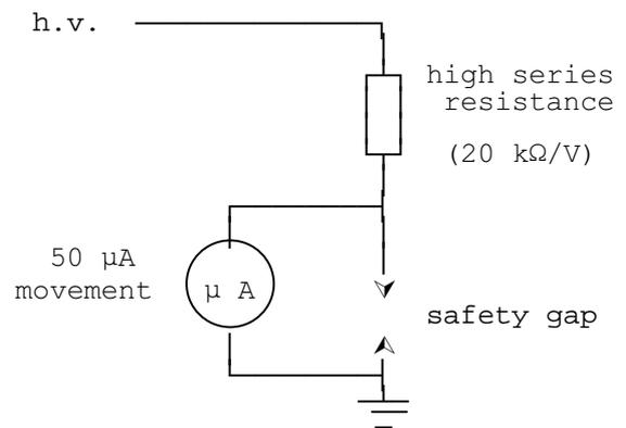
Figure 6.10 - Series resistor microammeter
