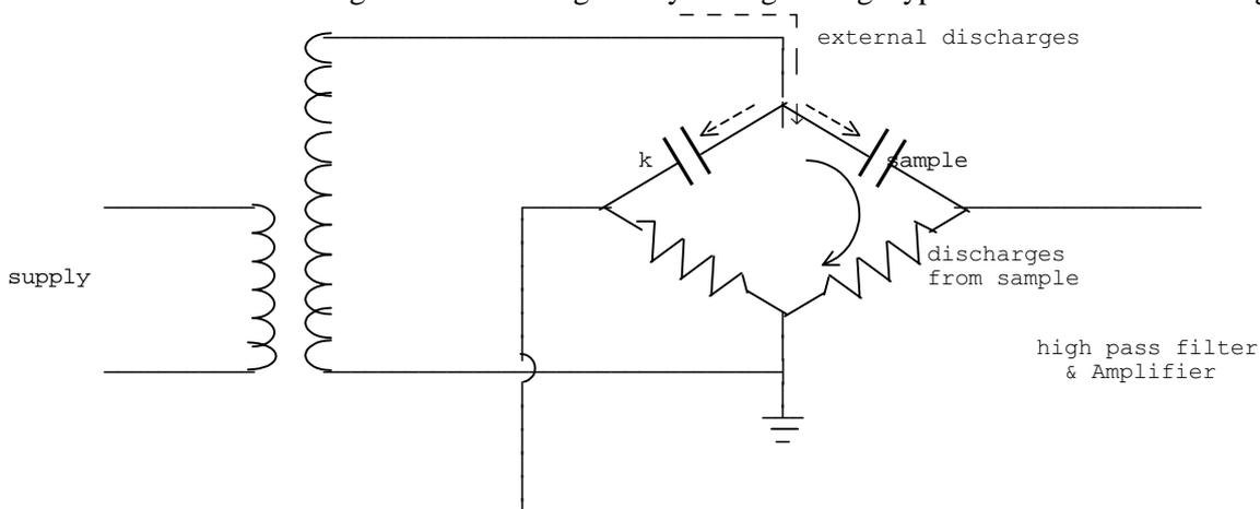
Figure 6.51 - Circuit to avoid effects of external discharges
