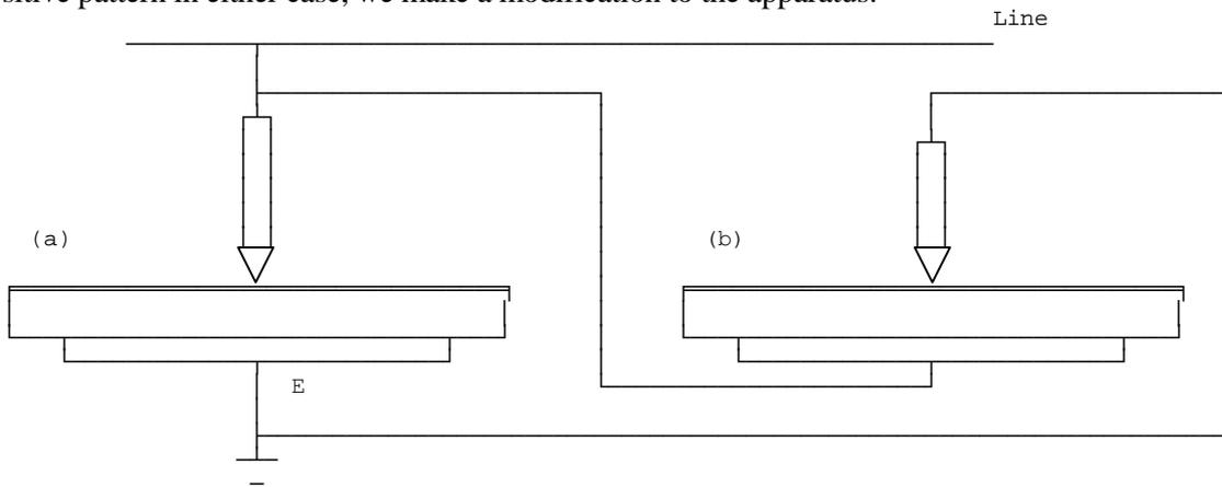
Figure 6.29 - Klydonograph for measurement of both polarities
