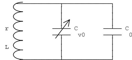
Figure 6.54 - Equivalent circuit for case (i)
