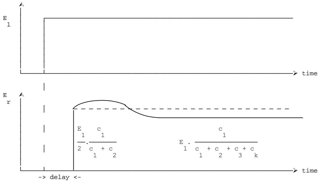
Figure 6.24 - Waveforms for split capacitor connection
