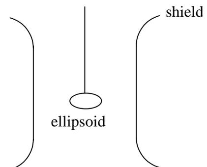
Figure 6.58 - Dumb-bell voltmeter
