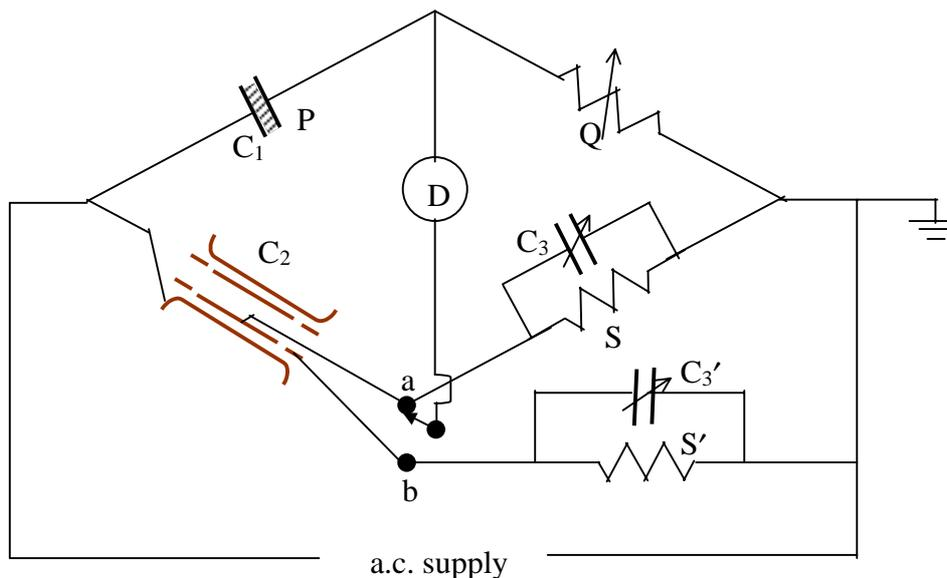
Figure 6.37 - Bridge with guarded standard capacitor
