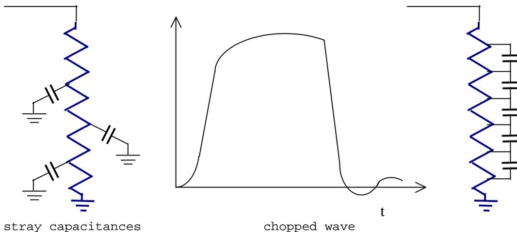
Figure 6.20 - Stray capacitances and chopped wave
