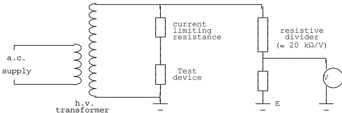
Figure 6.11 - Resistive potential divider method
