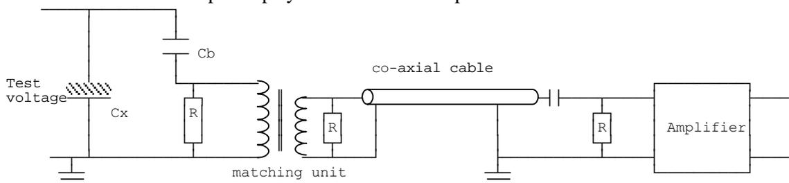
Figure 6.43 - Discharge detector input circuit
