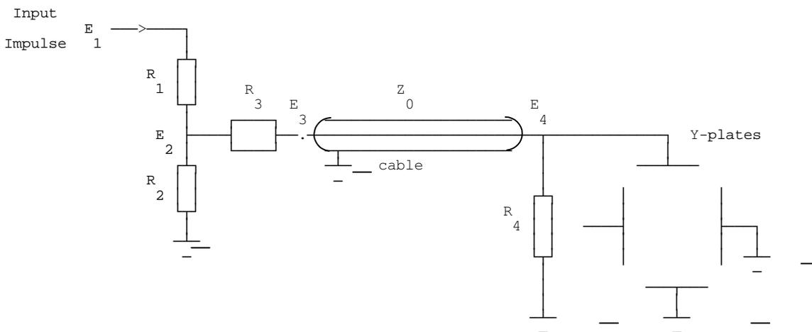
Figure 6.19 - Matching of resistive divider at both ends
