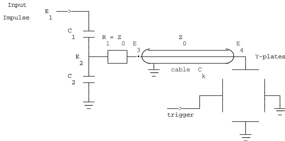
Figure 6.21 - Matching of capacitive divider (simple capacitor connection)
