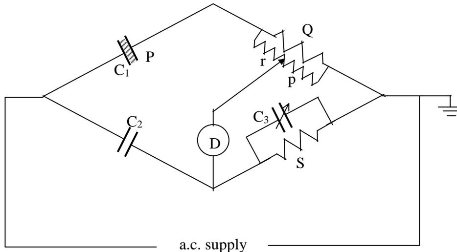
Figure 6.38 - Schering Bridge for high capacitances
