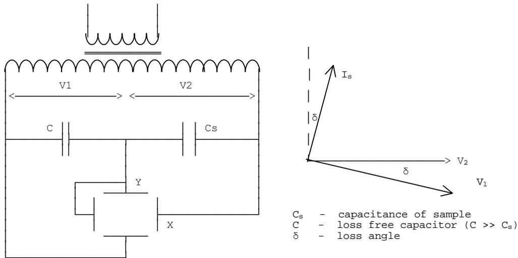
Figure 6.39 - Dielectric loss measurement using oscilloscope
