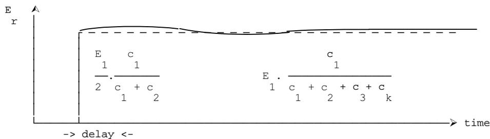
Figure 6.25 - Waveforms for split capacitor connection (low distortion)
