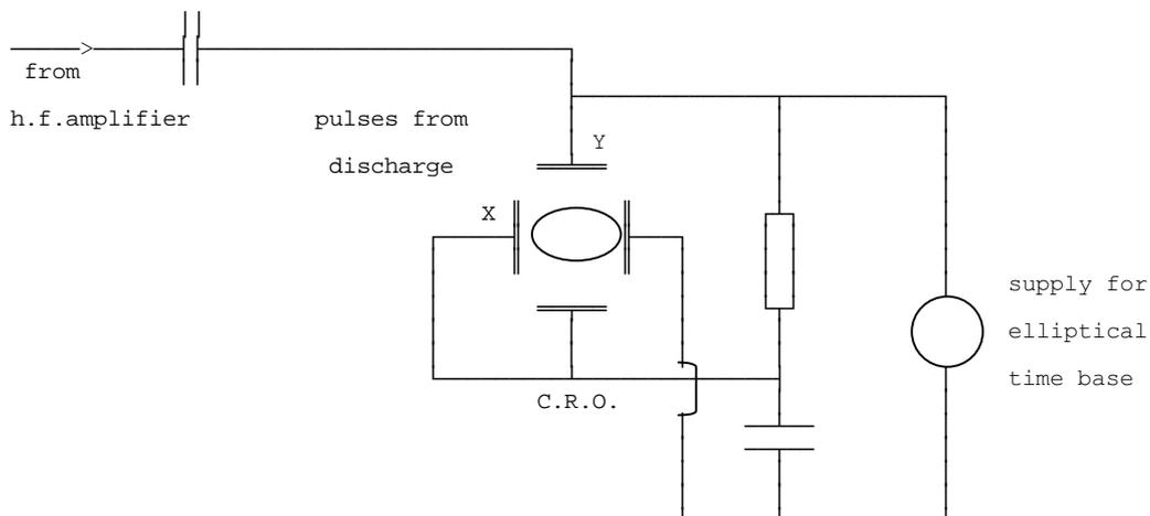
Figure 6.45 - Generation of elliptical time base
