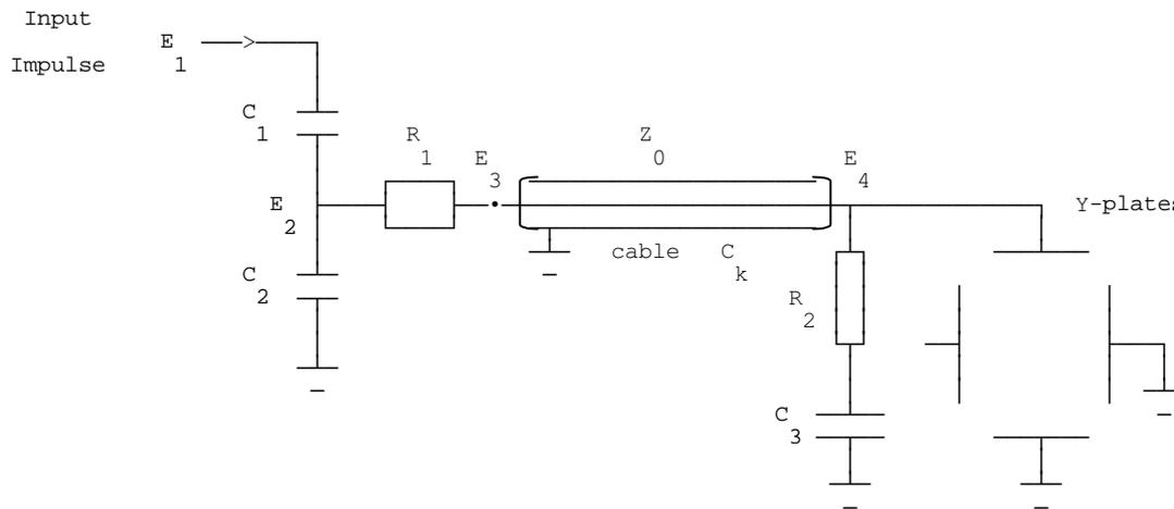
Figure 6.23 - Matching of capacitive divider (simple capacitor connection)
