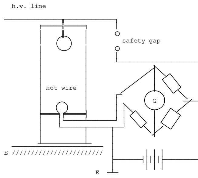
Figure 6.57 - Ionic Wind Voltmeter
