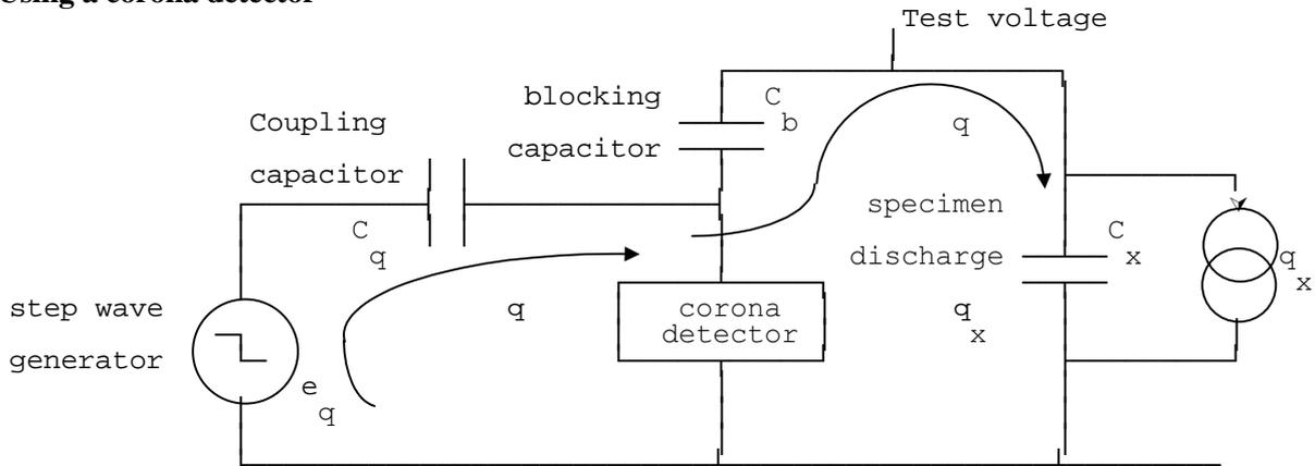
Figure 6.40 - Discharge detection using corona detector
