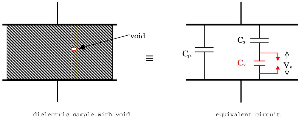
Figure 6.46 - Equivalent circuit of dielectric with void
