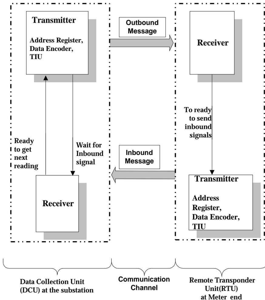
**Figure 1** Components of the Basic Communication System
