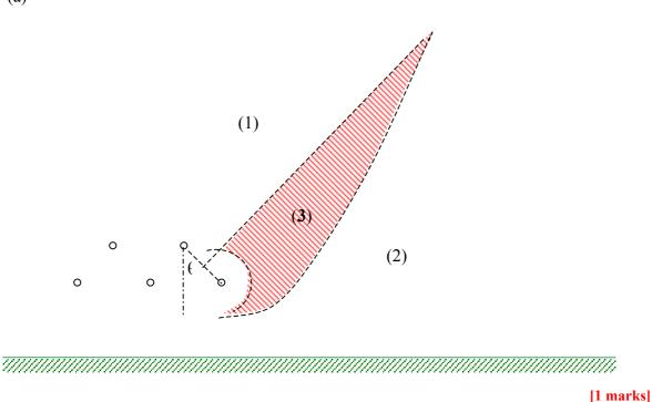
Figure shows the earth wire coverage of a transmission line against direct strikes.
