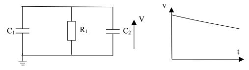
giving a discharging time constant  $1/\alpha = R_1 \cdot (C_1 + C_2) = R_1 \cdot C_1/\eta$
