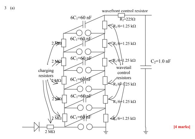
(b) During wavefront, since  $R_1 >> R_2$ , the approximate charging circuit is
