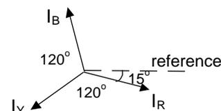
22. A 400V, 50Hz, 3 phase supply has a balanced load taking a line current of 3.0 A at a power factor of 0.8 lag. The total three phase power is equal to..1.663 kW..and the total apparent power is equal to..2.078 kVA...
