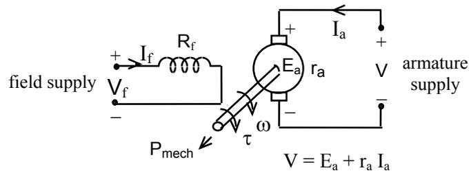
Figure 3 - Circuit model of a dc motor
