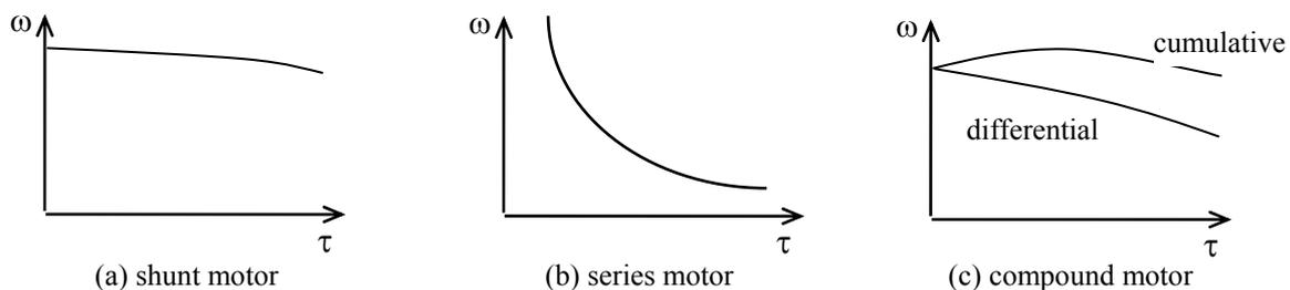
Figure 5 - Speed-torque characteristics of dc motors
