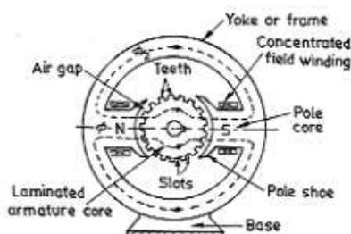
Figure 2 - two-pole dc motor
