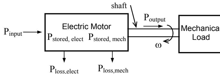
Figure 1 - Power flow in an electric motor
