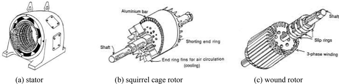
Figure 6 - rotor construction of induction motors
