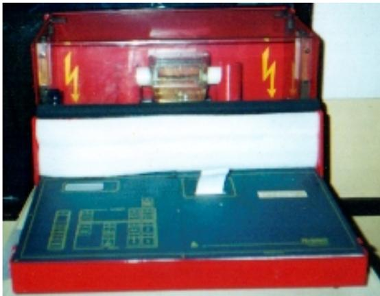
Figure 1 - Dielectric Test Equipment
