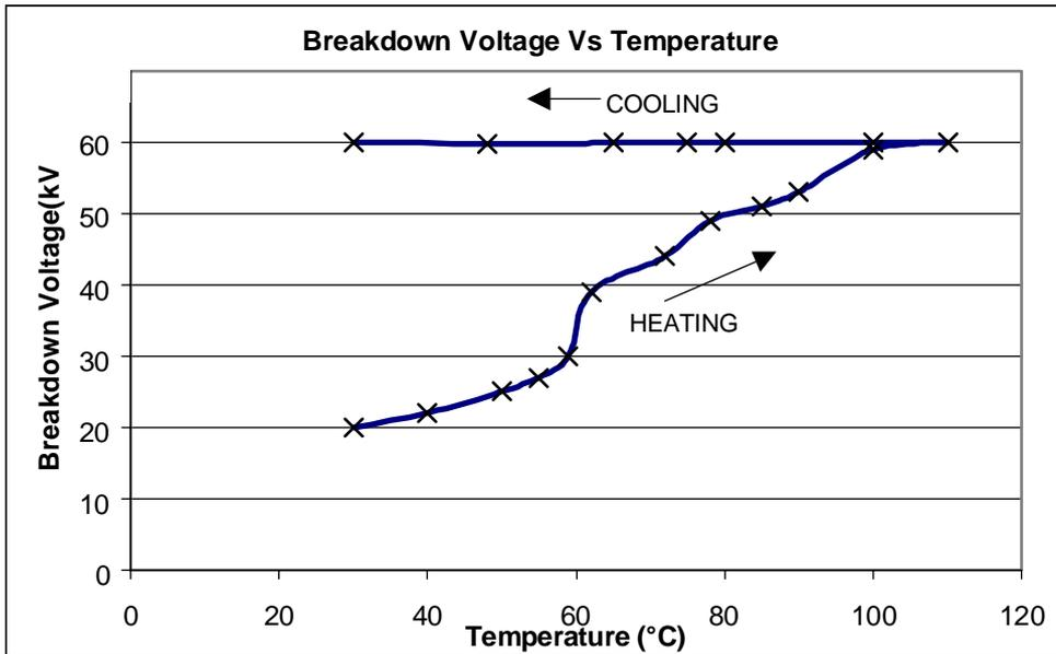
Figure 2 - Heating/Cooling Curve of Coconut Oil.
