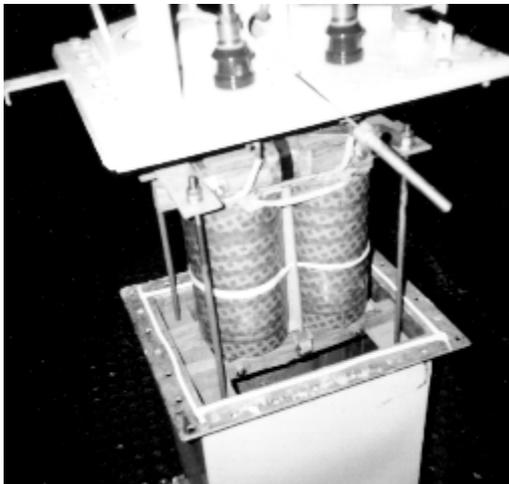
Figure 11 - Single Phase Coconut oil filled transformer
