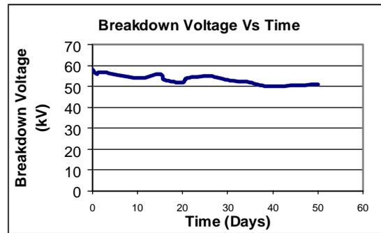
Figure 10 - Degradation of oil
