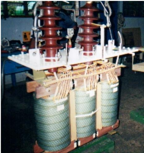
Figure 5-Core and Winding Assembly
