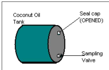
Figure 9 - Tank with seal cap opened
